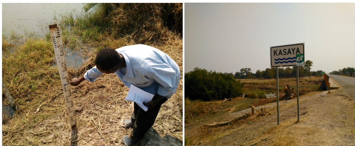
Figure 8. The gauge reader at the Kasaya Bridge takes river level readings three times daily for the Water Resource Management Authority.
