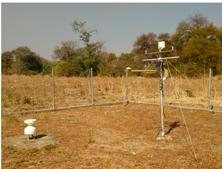
Figure 6. Automatic weather station in Sikaunzwe, which sends data directly to the ZMD, but is not disseminated locally.
