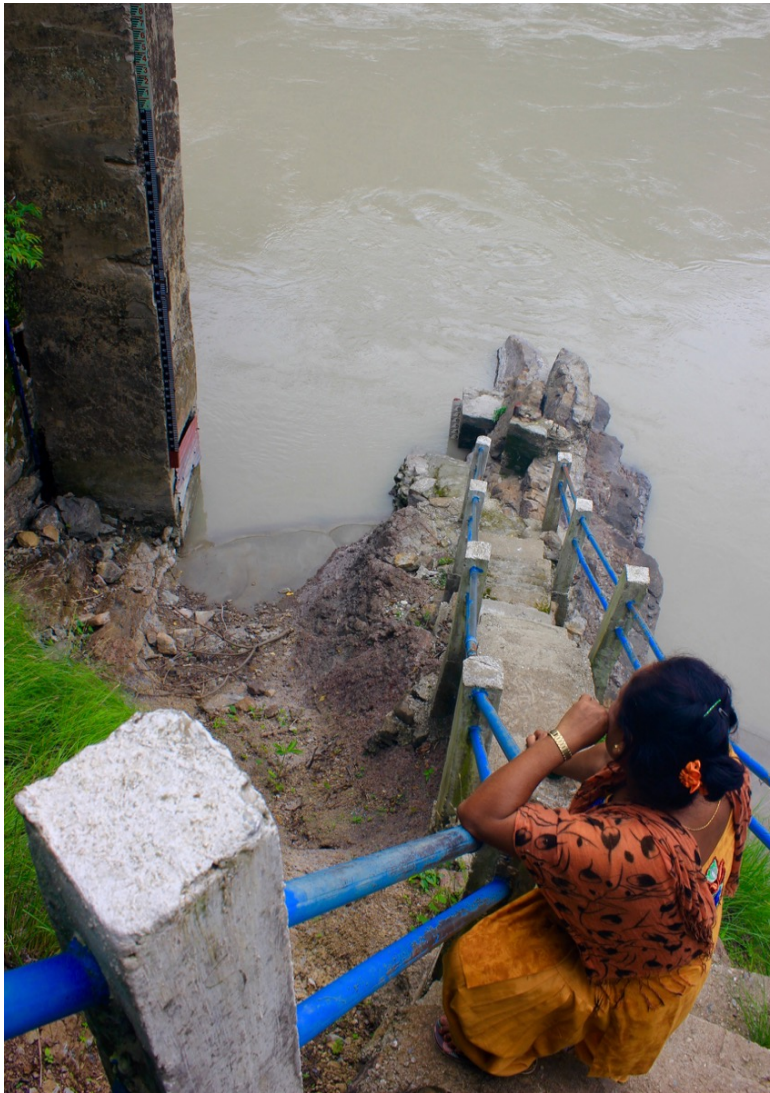
Figure 33. Prabati Gurung, a gauge reader employed by Nepal's Department of Hydrology & Meteorology, observes the Karnali River's water level at the Chisapani gauge station.
