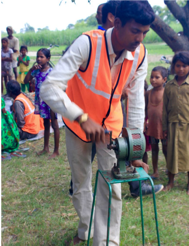
Figure 35. An example of a hand-operated siren used within villages to alert and mobilize residents when an early warning is received by the gauge reader in Chisapani.
